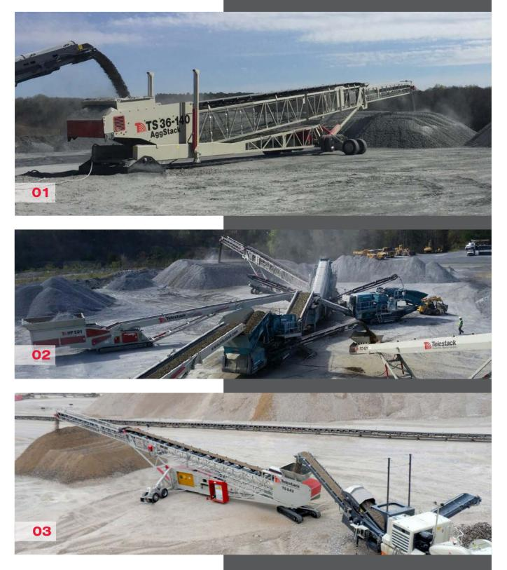
The Radial Telescopic units are fully mobile with optional tracks and integrated genset for ultimate flexibility when operating with mobile equipment.
