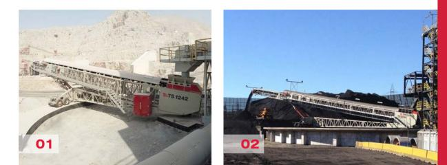
The Radial Telescopic units can easily integrate into a fixed plant system to ensure a quality finished product and large stockpile capacity reducing dust segregation, degradation, contamination and compaction of the material.
