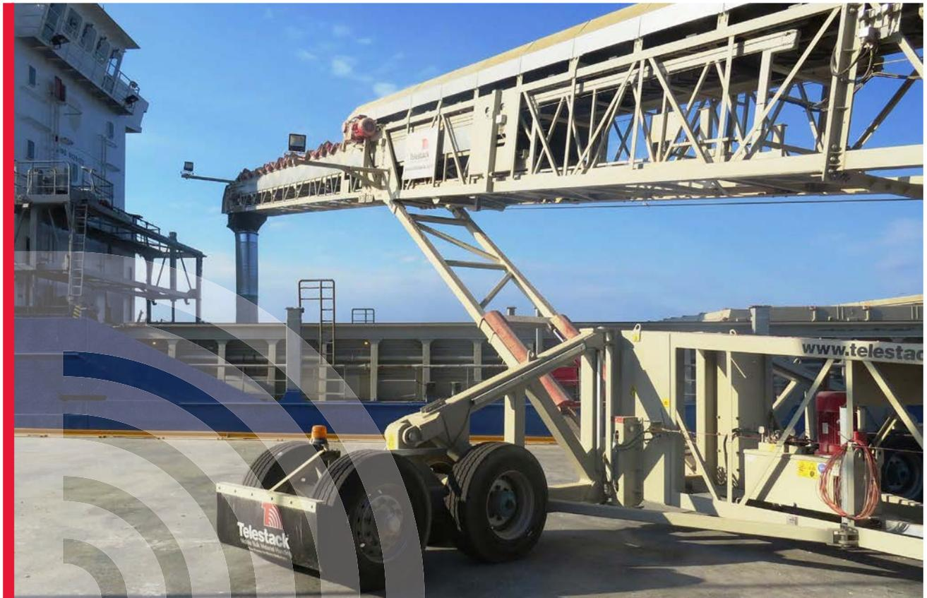
Telestack offers a wide range of mobile ship-loaders to load barges, coasters and larger vessels. Telestack's unique range of ship-loaders are designed taking into consideration maximum free-board heights, beam and quayside widths.
