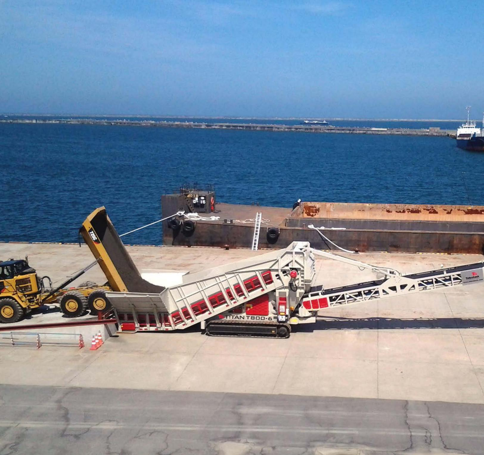
Titan T800-6 & TS 42 Export Radial Telescopic Shiploader bargeloading
