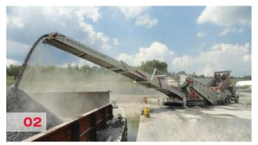
Telestack offer a range of solutions for feeding shiploaders directly from trucks, wheel loaders or grabs, taking into consideration the limited quayside space available when loading these types of barges and coaster vessels. The direct loading equipment ensures the material is transferred from quayside to vessel as efficiently as possible, eliminating the double handling of material.
