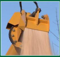
Rotating discharge chute for top loading of trailers and 290° rotation for broadcast chip spreading minimize truck relocation during loading. Available in straight, flexible, or vertical configurations. \*Pictured in vertical.
