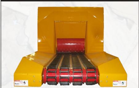
Larger feed opening, lower winged side walls, sloped deck, and reverse pivoting feed yoke make feeding brush and tops easy.
