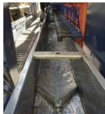
Picture showing open filtrate system, Terex Aquaclear filter press also available in closed filtrate configuration.
