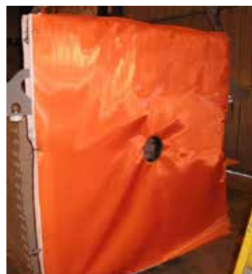
High quality mono nylon 6.6 cloth, with excellent cake release and abrasion resistance for long service life.
