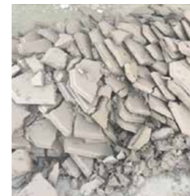
High pressure design leads to faster cycle times and dryer filter cakes which are more easily handled.
