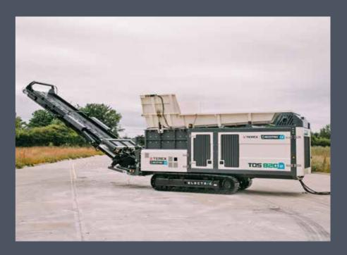
and noise the TDS 820e replaces the Scania DC13 diesel engine with a powerful 280kW WEG electric motor. This change also results in reduced maintenance time and costs. The TDS 820e is fitted with a small 55kW CAT C2.2 engine for tracking and machine set-up, resulting in minimal down time.
