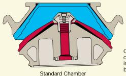
Changing crushing chambers only requires installing manganese bowl and mantle.
