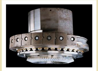
Due to the tighter tolerances of the wedge plate's roller bearing's —1/10 those of a bronze-bushing cone—a true setting is maintained. The tighter tolerances reduce oversize to about 20% instead of the 50% as with bronze-bushing cones when making a 1/2" (12.7 mm) minus product. This allows more feed material in the circuit with less recirculation and that means more production.
