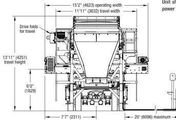
Unit shown with the following options: extended walkway along chutes, hydraulic power for roll-away chutes, removeable switchgear panel, and hydraulic leveling jacks.
