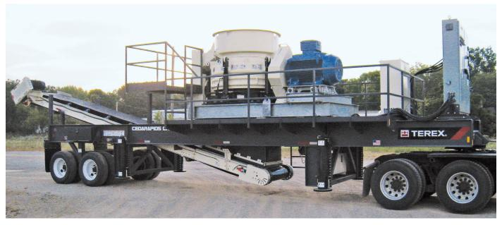
Unit shown with optional electrical switchgear panel, power cables, and hydraulic run-on jacks.
