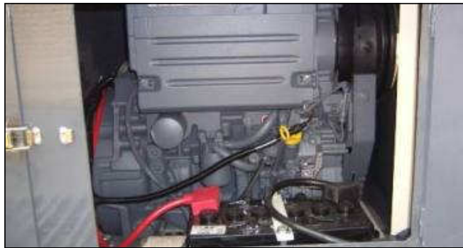
Deutz 4 Cylinder TURBO D 2011 50Kw (68HP)
