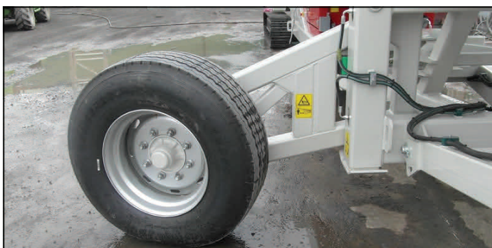
Internal hydraulic radial wheel drive (Radial movement)
