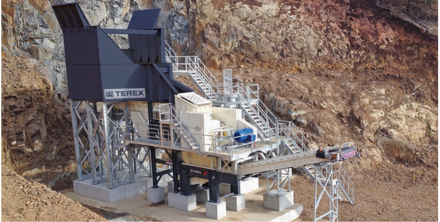
Unit shown with optional hopper wings, hopper extension, extended length discharge conveyor, and rock breaker structure with walkways.
