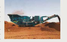
\*Depends on application Engines are available that are certified to US EPA and EU off road diesel emission standards. Talk to your dealer about possible certification options (i.e. Tier 3/Stage 3A:, Tier 4i/Stage 3B:, Tier 4F / Stage 4). **Side Conveyor (option)** Width: 800mm (31.5") Discharge height: 3.6m (11' 10") Tracks Width: 500mm (15.7")
