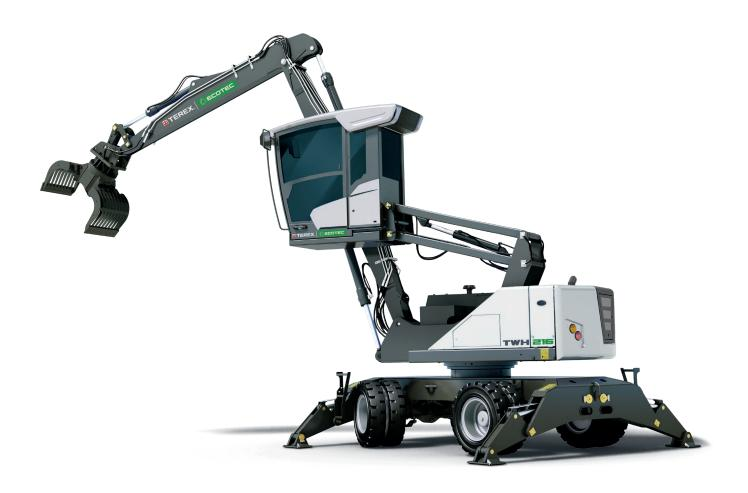
85 kW (Diesel, EU Stage V / US EPA Tier 4) 75 kW (Electric) 14.6-17.1 t
