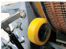
4WD for the drum screen, this concept doesn't only considerably reduce abrasion and maintenance effort, it also enables drum change in record time and without tools.
