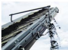
The side conveyor as well as the rear conveyor are offered in two different lengths and are available in 3.500 mm and 5.000 mm.
