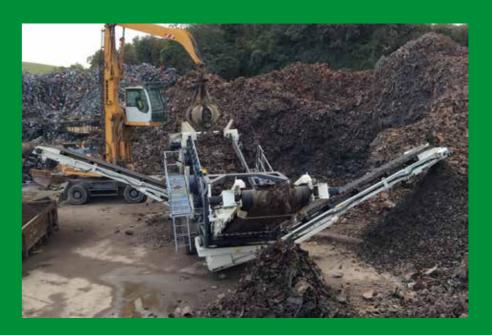
Terex® Ecotec's tracked heavy duty screen can be operated in a wide range of primary and secondary screening applications. The TRS 550 Recycling Screen features a two-deck German-designed recycling waste screen with Flip-Flow-Screen technology. This high-performance waste screen is combined with advanced technology on the bottom deck to elevate the TRS 550 into a class of its own.
