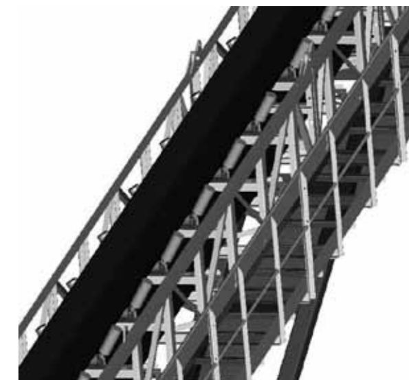
60° side rollers for minimum spillage and maximum capacity
