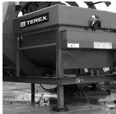
Jacking legs and towbar for quick transport and setup
