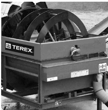
Weir on front of machine for maximum silt removal
