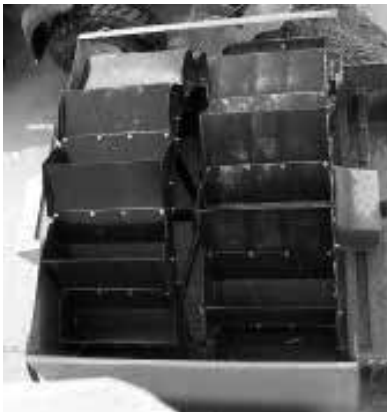
Twin buckets allows one or two final products
