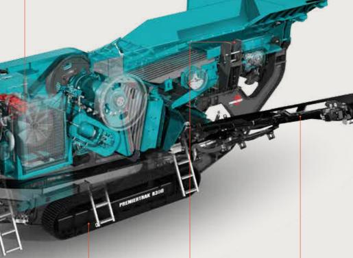
**Power Unit** Tier 3/Stage 3A: Width: 400 mm (15.7") CAT C9 205kW (275hp)
