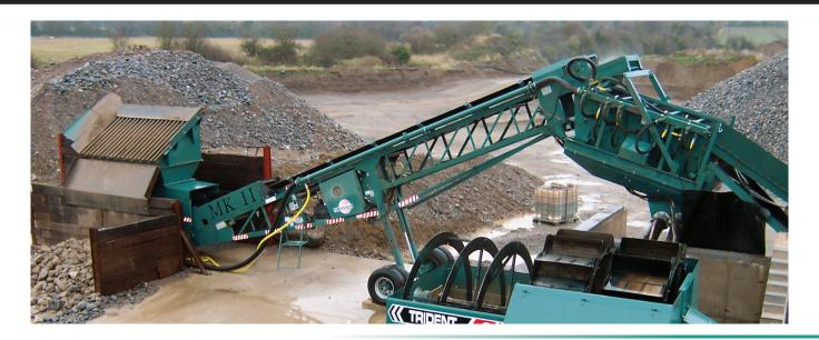
The Powerscreen® Mark II is a time proven entry level mobile screening unit that is portable, easy to setup and maintain. Ideal for smaller end users who require a affordable flexible product suitable for applications such as topsoil, coal, crushed stone, recycling, sand and gravel.
