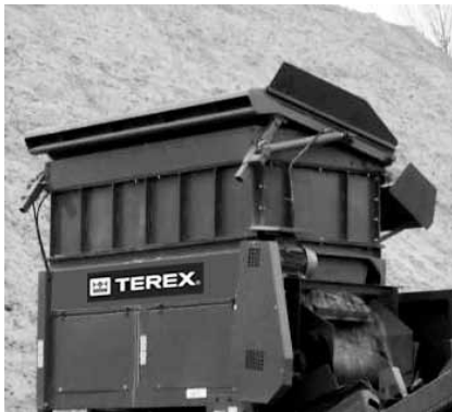
500 or 700mm hopper extensions available for increase capacity
