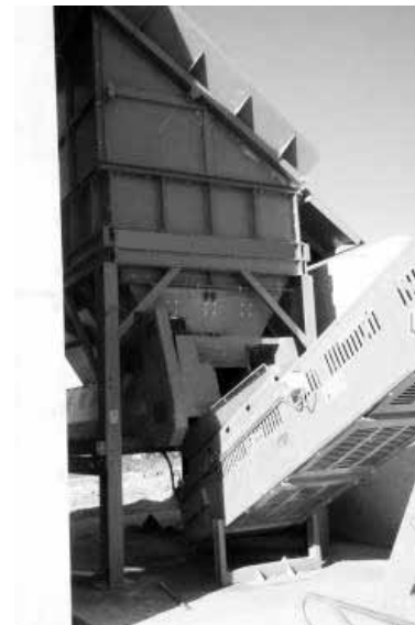
Extension to increase capacity
