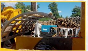
60" wide cleated discharge belt provides unrestricted discharge of ground product. Split hog box for ease of maintenance. The entire grinding chamber rises for quick tip and screen changes.
