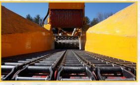
Infeed walls wing outwards to increase loading clearance and funnel material.
